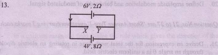
The figure shows a circuit with two cells in opposition to each other. One cell has an emf of 6V and internal resistance 2 ohm and the other has emf 4V and internal resistance of 8 ohm. Find the equivalent emf and internal resistance across terminals X and Y
